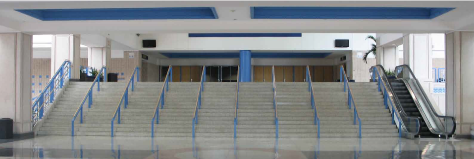
Left #32 and Right #34 Staircase — Total: 15 risers each 50'-6" w x 6 1/4" h
