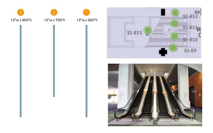
We recommend avoiding light color backgrounds in the design due to black particulate created by the escalator handrails settling on the runners.
