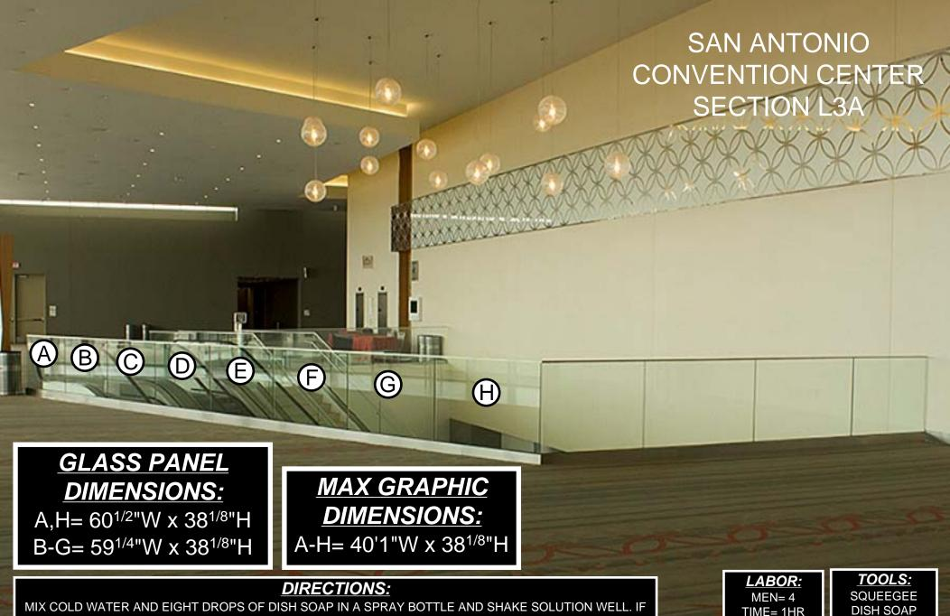
NEEDED, CLEAN SURFACE OF GLASS WITH WINDEX AND TOWEL FIRST. NEXT, SPRAY GLASS AND GRAPHIC WITH A LIBERAL AMOUNT OF SOLUTION BEFORE APPLYING GRAPHIC TO THE GLASS. LINE UP AND LEVEL OUT GRAPHIC ON GLASS. USE SQUEEGEE TO REMOVE SOLUTION FROM INBETWEEN GRAPHIC AND GLASS. WIPE THE GRAPHIC CLEAN OF SOLUTION RESIDUE BEFORE MOVING TO NEXT JOB.
